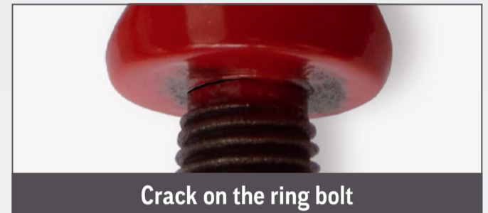
Damaged wire rope connection
